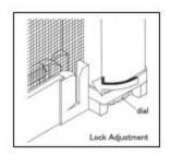
\*The positions of the Lock Adjustment and the Spring Adjustment are up-side-down on the right side screen and the left side screen.
